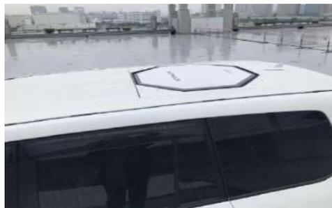
Fig. 8. The 70 cm integrated terminal installed in the roof of a Toyota Land Cruiser.
