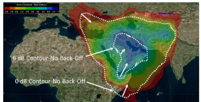
Fig. 6. SNR coverage map for the 70 cm vehicle terminal operating on IS-17
