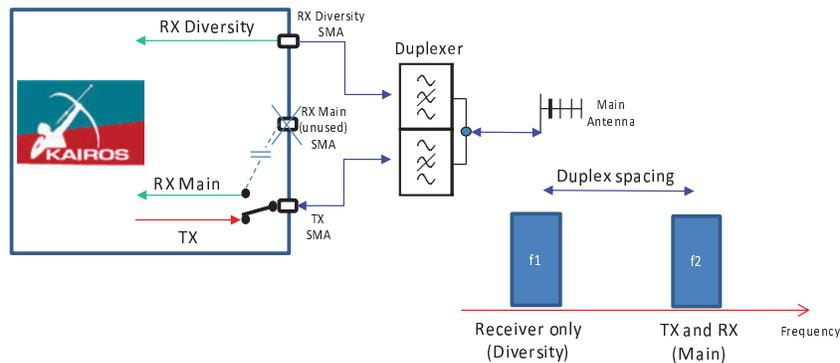
This realization allow to operate like a normal duplex station on  $f1=f_{rx}$  and  $f2=f_{tx}$ , and also in simplex/direct mode at  $f2$ . The soft diversity feature, obviously, in this special application is lost. More details can be asked to Factory.
