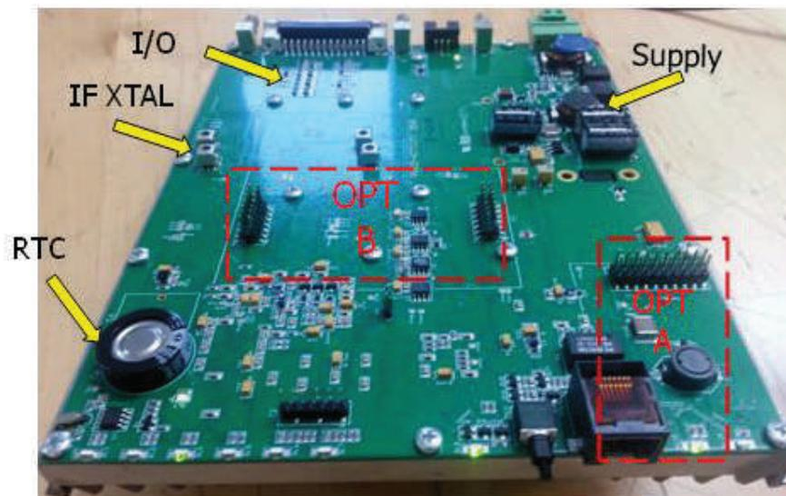
The option boards are automatically detected and recognized at the equipment power on.
