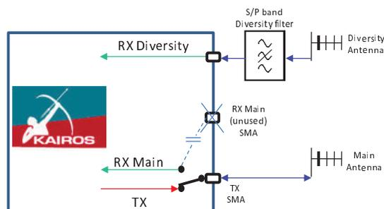
The internal isolation between the Diversity channel and the TX is around 80dB. This allow special realization like a duplex/simplex station:
