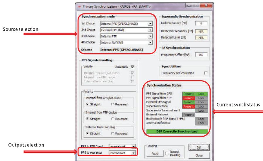
In multi equipment assembly like a multicarrier trunking application, it is possible to use only 1 GPS receiver shearing the PPS signals to the other equipments via the 6pin connector placed in the back of the equipment as shown in the following paragraphs.
