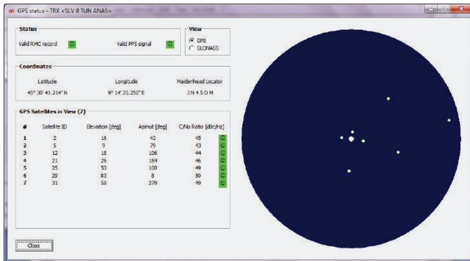
The PPS acquire time is around 1 minute with good GPS signals (the frontal led "RX1" flashes red until the PPS is ready). Once the PPS is acquired (the frontal led "RX1" flashes orange), another minute is request to synchronize in time and frequency the equipment (than the frontal led "RX1" flashes green synchronously with the arriving PPS).
