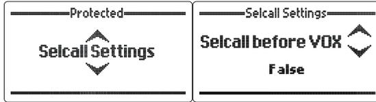
The Selcall before vox feature of the 2060 telephone interconnect allows the telephone operator to begin voice communications with the HF network immediately without having to send a Selcall first. There are 2 settings available:
