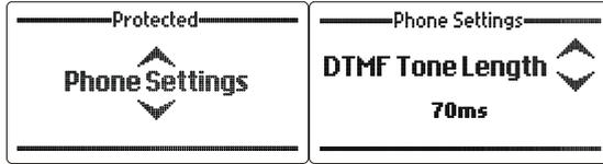
This is the length of one DTMF tone. This is only effective when tone dialling is selected. The time is measured in milliseconds.
