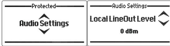
This section sets the transmit audio level to the local transceiver, 0dB is the default.
