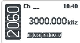
Enter the channel number required using the numeric keys, channel range is from 1 to 9999 inclusive. **Note:- Channel zero cannot be selected.** (example selects channel 12)
