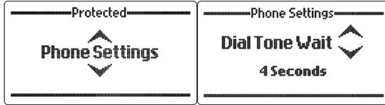
This is the period to wait for before determining if a dial tone is present. The time is measured in seconds. Dial tone checking can also be disabled.
