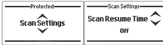
This section sets the time period after which the 2060 will automatically resume scanning from the last operation i.e. key press or PTT. The scan resume time period can be set between 1 and 30 minutes or it can be disabled.
