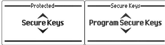
This allows the operator to view secure call keys for different Selcall IDs.
