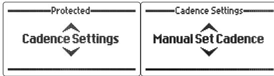
This feature allows the operator to manually enter the busy and ring cadences on non-country specific telephone networks. All tones can be set from 0 to 9999 milliseconds. Busy tones let the operator set the busy on and off times, ring tone allows the operator to set 2 on tone lengths and 2 off tone lengths. The example below will set up a busy on tone length.
