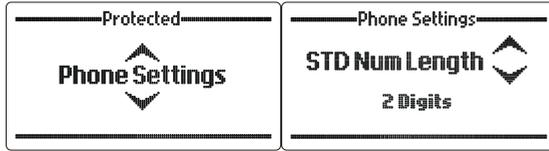
This option will set the number of prefix digits required to calculate if the telephone number dialled is in fact a STD number. One to four digits can be selected.
