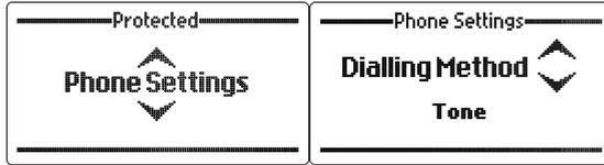
Dialling method selects whether the telephone exchange uses pulse or tone dialling.
