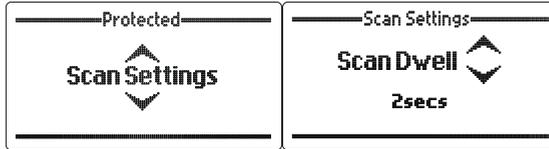
Selects the length of time the 2060 dwells (waits) on a channel after scan has been stopped after a Selcall signal has been detected. The dwell time can be set from 1 to 10 seconds.
