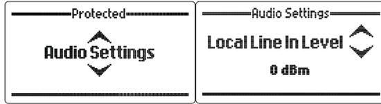
Sets the receive audio level from the local transceiver, the lower the level the higher the line amplifier gain.
