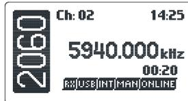
Once the number is dialed and answered the 2060 shows the call length in the bottom right hand section of the screen. This means that the HF transceiver and the telephone user are now able to communicate to each other.
