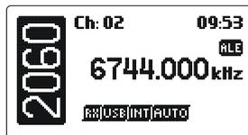
**Checking for the best channel to use between two stations - Beacon Call**
