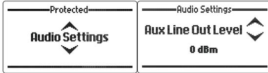
This section sets the transmit audio level to the auxiliary connector, 0dB is the default.
