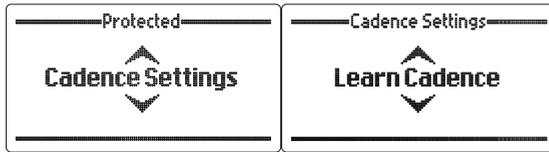
This feature allows the 2060 interconnect to learn busy and ring cadences on non-country specific telephone networks by sampling on line signals. The 2060 allows the operator to enter telephone numbers to dial so that ring and busy signals can be sampled. For the 2060 to operate at optimal level the busy and ring tones generated from the dialled numbers must be correct.
