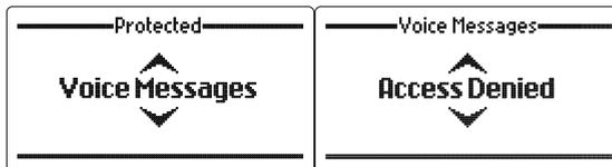
The "Access Denied" is played on air to the HF network or online to the telephone user when a Selcall ID without the correct level of security is accessed. (Selcall, Telcall etc....).
