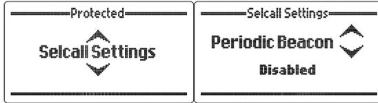
The periodic beacon feature of the 2060 telephone interconnect allows beacon tones to be transmitted by the interconnect at a set period of time on each programmed channel. This gives HF station operators the ability to know if an interconnect is available and also signal quality. The period can be set from 1 to 60 minutes at intervals of 1 minute, or the beacon can be disabled.
