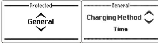
This section allows the call charging method to be set. This is used to calculate charges for phone calls. Done either by a time connected method or using the different types of PSTN charging pulses that are generated on the phone line by some telephone exchanges. -
