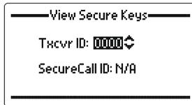
The operator can use the **Scroll keys** to scroll to the Selcall ID required for viewing, or the operator can enter the Selcall ID
