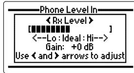
Adjust the receive gain by using the left and right arrow keys, level should be set within the "Ideal" area. Once the correct level has been
