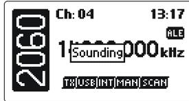
"Beacon Call" allows the operator to determine the signal quality between their interconnect and a station on a particular channel and vice versa.
