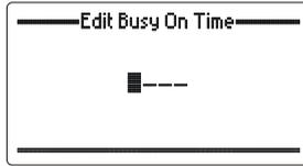
Enter the required busy on time in milliseconds then press the
