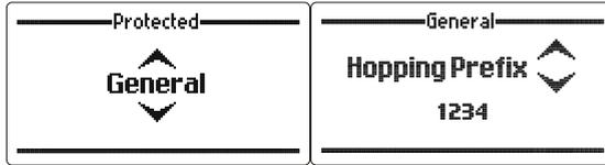
This section allows the interconnects hopping prefix to be set. This is used during secure calls between HF stations and telephone subscribers -
