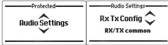
This setting tells the 2060 if the installation is for use in a local transceiver configuration or a local receiver remote transceiver configuration. Normally this is set to "RX/TX common".
