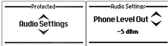
The audio level to line is set up in this menu. This level can be increased up to 0dBm for phone lines with loss. Typically, this level can be set to -5dBm for most lines.
