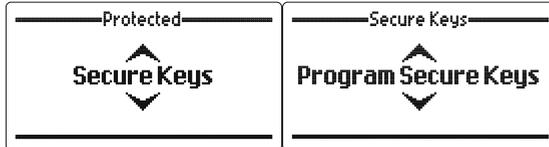
This allows the operator to setup secure call IDs for individual or groups of Selcall IDs.
