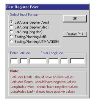
Select input format. Latitude and longitude values can be processed using any one of the three following formats:
