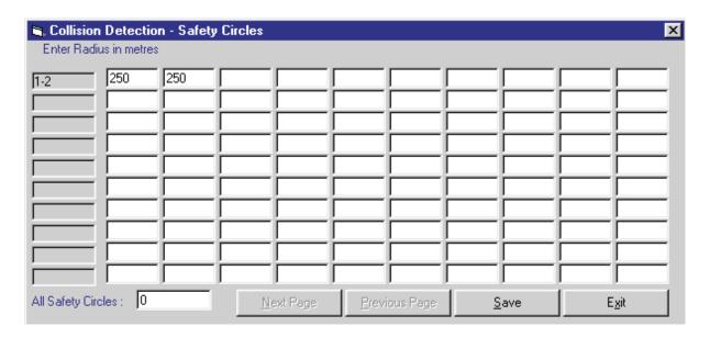
For every mobile ID a radius (m) can be defined, that creates an area around the mobile unit. This area is called a safety circle. If any mobile position falls inside another mobiles safety circle then an audible alarm is activated. Each mobile radius is entered individually or one radius can be assigned for all mobile units. Eg. Above ID's 1 and 3 have 250 metre radius.
