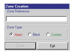
Select the required zone type from the zone creation window and enter a reference describing the zone and click the 'Create' button. To save the zone press <Enter> or the right mouse button. The maximum number of points in a zone is 50. The pointer changes to cross-hairs,(+). Using the left mouse button click on all of the points which define the perimeter of the zone to be created. To delete the previous point press the 'back space' key.
