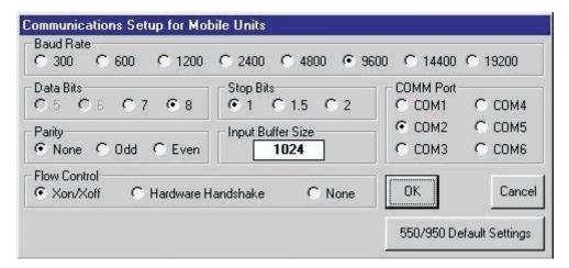
Allows setup communications to base transceiver, does not require changing as is defaulted to suit Barrett 550/950 Transceivers.
