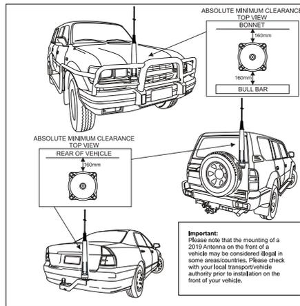
**Caution:-** Whilst the Barrett 2019 automatic tuning mobile HF antenna is designed to withstand vibration to military specifications on tired vehicles, some mounting positions on large prime-movers, particularly front mounted bull bars, are subject to vibration that far exceeds this specification. Do not mount the Barrett 2019 antenna in positions such as these as damage to the antenna may result.
