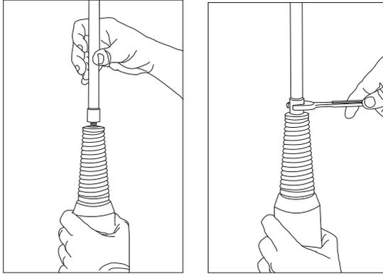
To mount the whip section it is recommended that only one section of the whip is screwed onto the antenna at a time. The whip section should be hand tightened fully then a suitable tool (ie: a spanner) can be used to tighten the section a further 10 to 20 degrees clockwise while holding the antenna body with a free hand.
