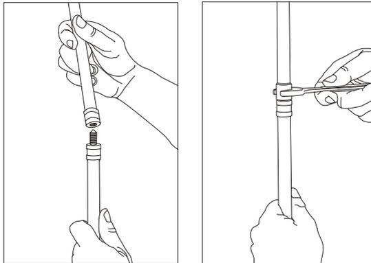
To mount 2 whip sections together the unattached whip section should be hand tightened fully then a suitable tool (ie: a spanner) can be used to tighten the section a further 10 to 20 degrees clockwise while holding the already screwed on whip section with a free hand.
