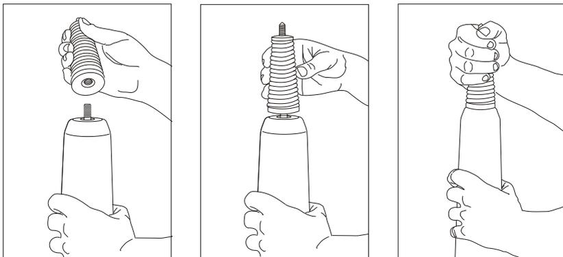
The base spring should only ever be hand tightened, if a tool is used it may damage the spring base.
