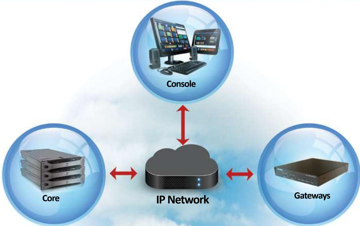
The **AcomNOVUS Core** is based on commercial-grade server technology. It utilizes a cluster arrangement with stacked switching equipment to provide a completely redundant solution that keeps your communications up and running reliably at all times. It is highly energy efficient, has a "small footprint," and can be either centrally located or separated for geographical diversity.
